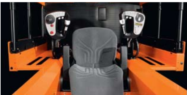
The twin control panels allow easy access to the forks for order picking
