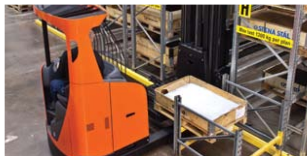
The VRE125SF's shuttle forks allow the narrowest aisles, for maximum use of space
