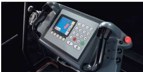
The A-series' integrated control panel provides electronic access to all truck functions
