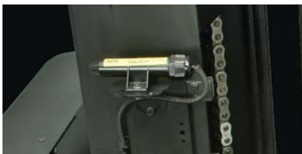
The new load camera option supports faster load handling by giving the operator a clear view of the load from above. A fork-level camera is also available
