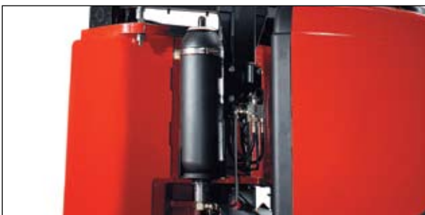
The BT Advanced Lifting System means that the lift motor works to lift little more than the load itself
