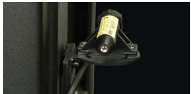
The optional aisle camera provides the operator with a clear view of any obstructions in the aisle that may not be visible from the cab
