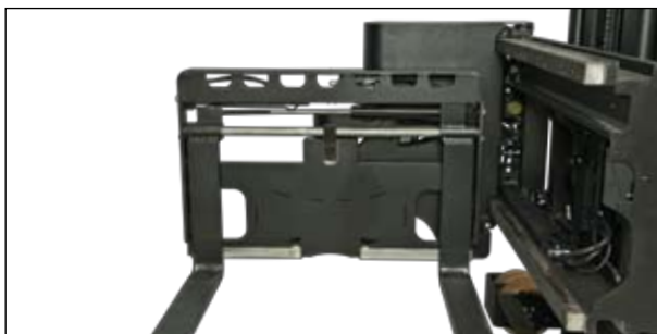
Autorotation (option) allows the operator to rotate and traverse the forks simultaneously with one lever. The action is automatically configured to take the minimum space possible
